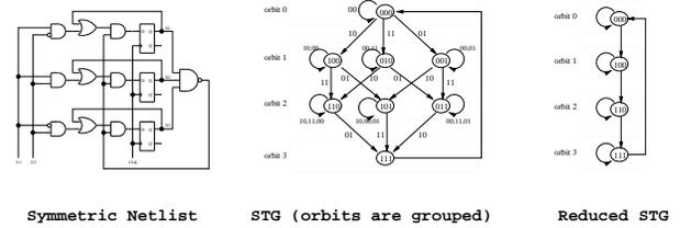
Figure 2: A symmetric netlist, its STG, and reduced STG. The orbits are the circled sets of states.
