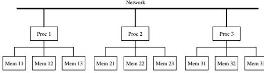
Figure 1: Multiprocessor network with groups of symmetry.
