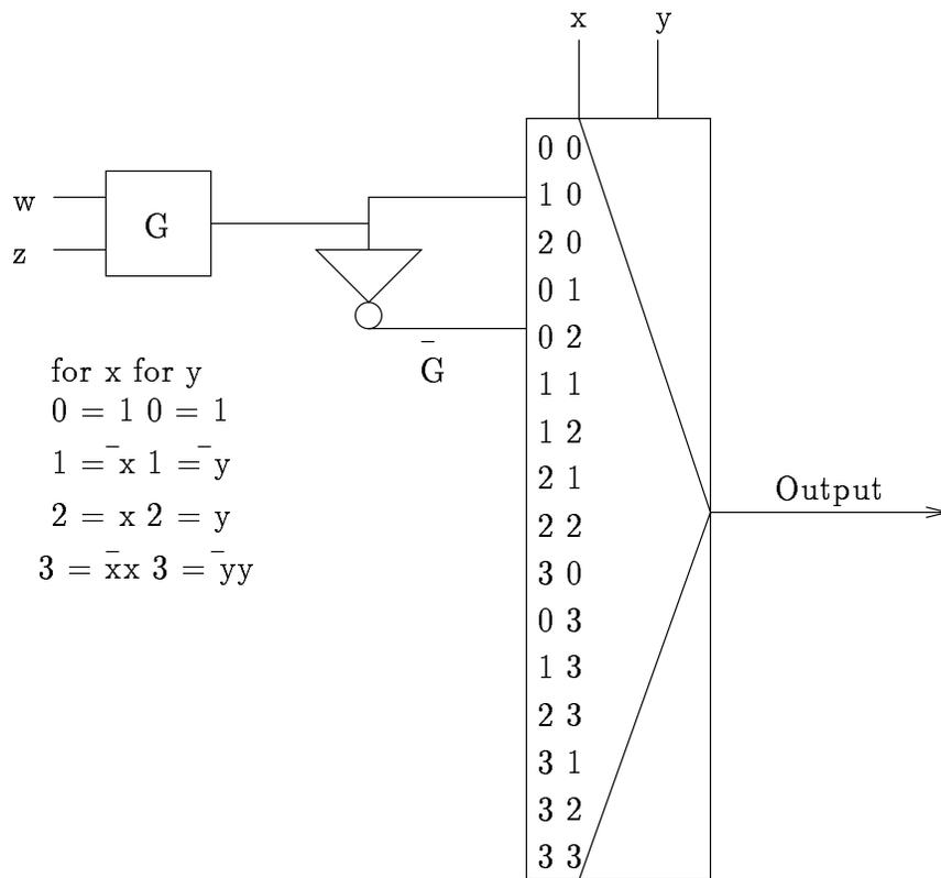
Figure 31: A Decomposition of a Fuzzy Function from Example 19.5 using a Fuzzy Multiplexer.
