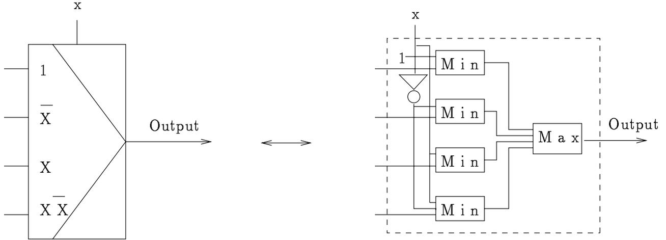
Figure 30: Fuzzy Multiplexer, (a) symbol, (b) internal structure using a Fuzzy Inverter, Min, and Max gates
