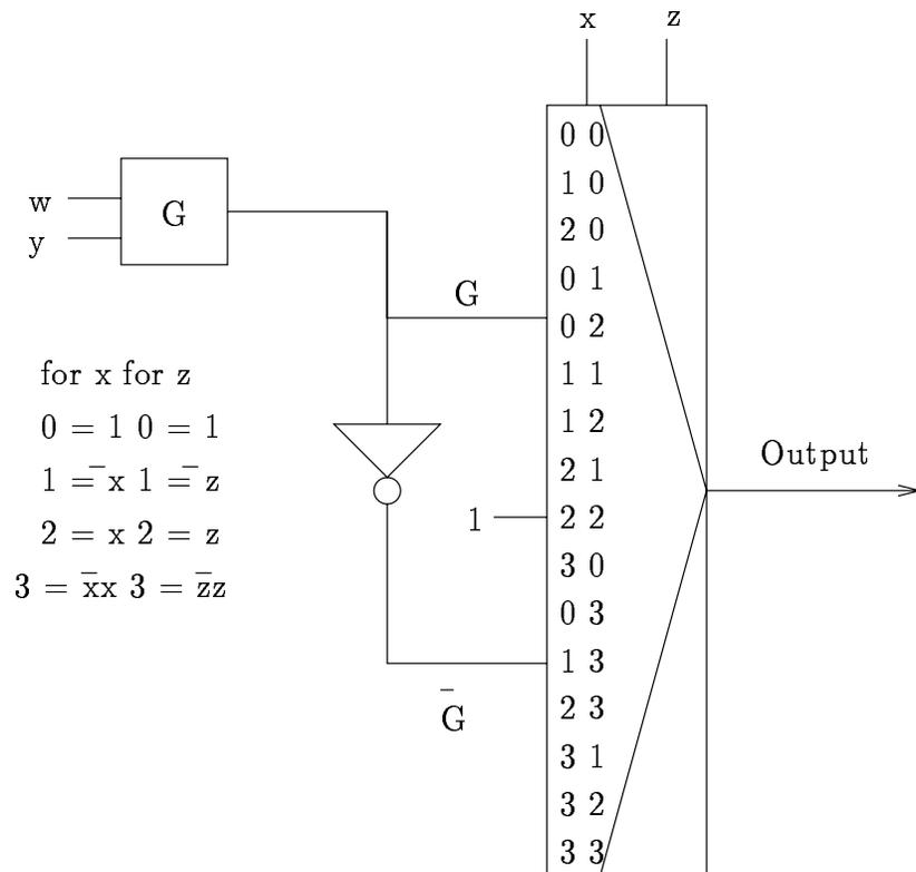
Figure 41: The decomposed fuzzy circuit
