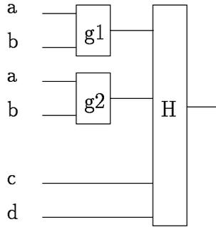
Figure 16: Two-output predecessor block in serial decomposition
