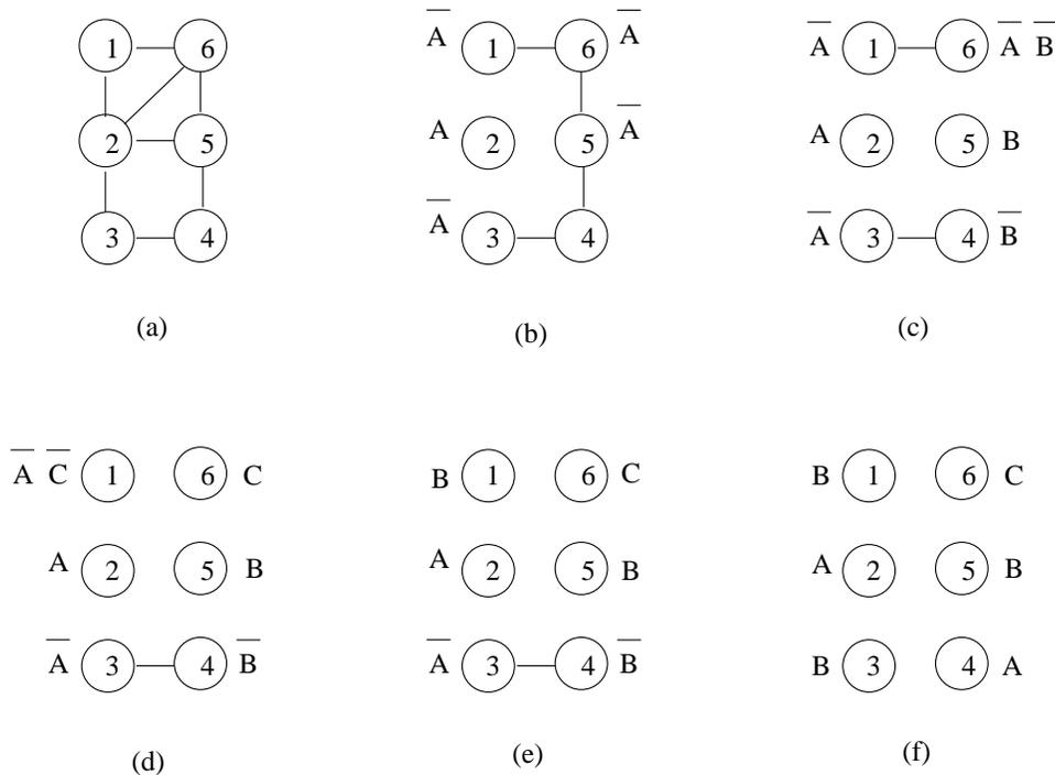
Figure 65: Graph coloring using Color Influence Method
