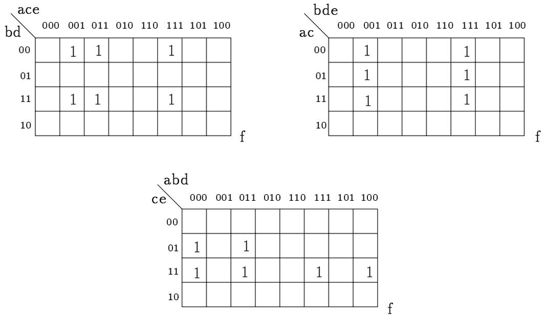
Figure 63: Partitions after variable partitioning
