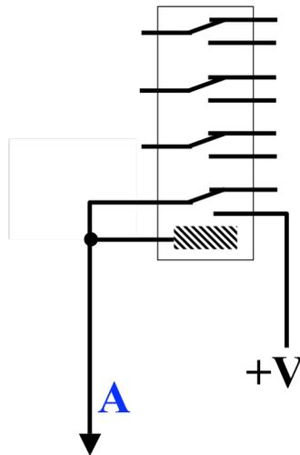
If line “A” should ever go high, this relay will turn on. However, if “A” is subsequently disconnected to whatever was driving it, the relay will stay on, due to the feedback loop from
