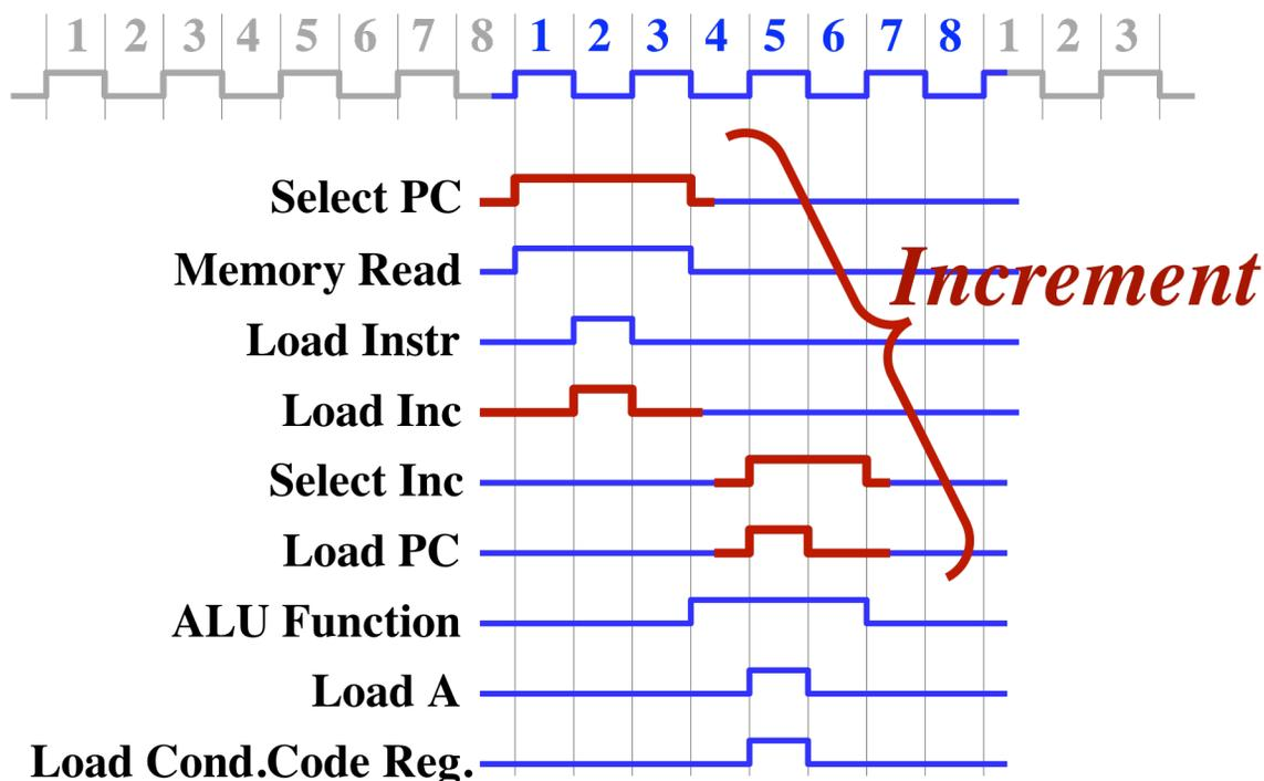
In the first step, we are gating the PC onto the address bus (Select PC) and loading the Increment Register (Load Inc). The Increment Register is loaded with the value on the bus, plus one. In the second step, we are gating the Increment Register onto the address bus (Select Inc) and loading the PC (Load PC).
