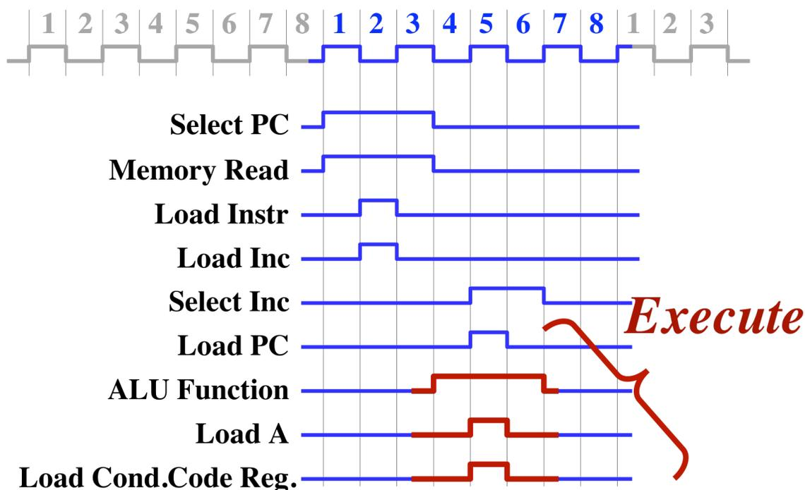
The B and C registers are always supplied to the ALU, so the ALU only needs the 3-bit function code, telling which operation is selected, to output the correct result onto the data bus.
