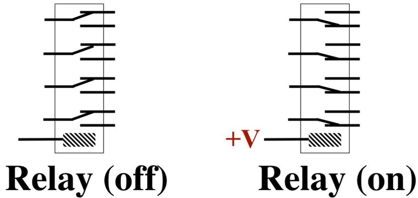
Normally, relays are drawn in the “off” position, but sometimes it helps in understanding a circuit to portray some relays in the “on” position.
