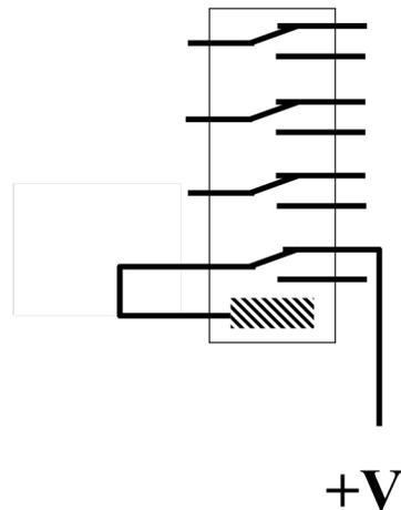
When this relay is off (as shown), power will be supplied to the coil, causing it to turn on. When the relay is on, power will be disconnected from the coil, causing it to switch off. The relay will oscillate as fast as it can, making a buzzing sound. The relays used here are rated for a maximum switching speed (5 cycles per second) and when buzzing, they will overheat and fail.
