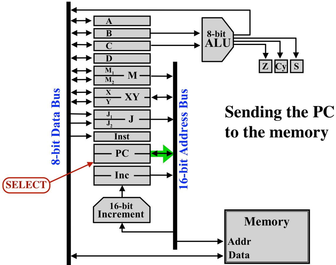
At the same time, the Mem-Read control line goes high. This gates the output of the static RAM onto the 8-bit data bus.
