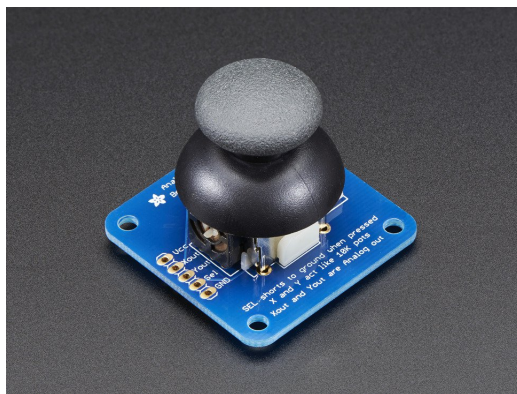
Figure 3: Photograph of the Adafruit joystick board, from www.adafruit.com . On the left of the image, 5 input/output pads with labels, Vcc, Xout, Yout, Sel and GND are visible. Vcc and GND are for DC power compatible with the analog inputs of the microcontroller, e.g., 3.3 VDC or 5 VDC. Xout and Yout are the potentiometer outputs, which are connected to analog input channels of the microcontroller. Sel is the momentary output button, which is connected to one of the interrupt channels on the microcontroller.
