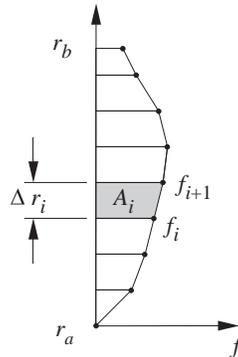
Figure 6.8: Trapezoid rule for numerical integration of the velocity profile.
