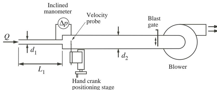
Figure 6.1: Apparatus for measuring flow downstream of a sudden expansion.
