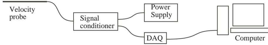
Figure 6.2: Data acquisition system for velocity measurements.
