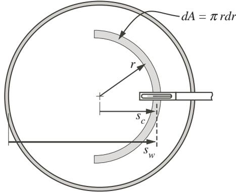
Figure 6.7: Coordinates used to indicate the probe position and integrate the velocity profile.
