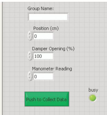
Figure 6.6: Partial view of the virtual instrument used to collect data. The input controls in this section are used to record the probe position, and the pressure drop.
