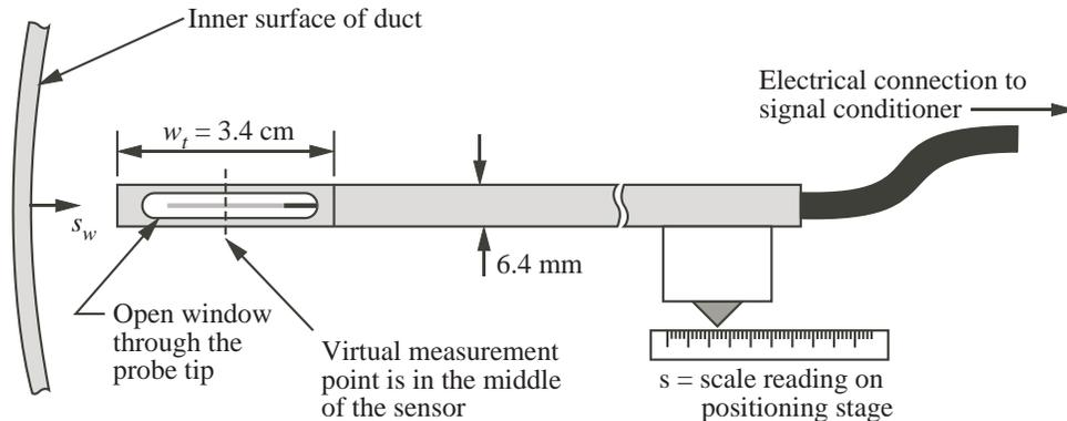
Figure 6.3: Detail of the velocity probe tip.
