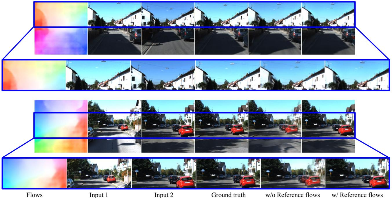
**Figure 7:** Effect of reference flows. By directly estimating dense flows and using them to guide the estimation of the target dense appearance flows and masks, our results avoid ghosting or blurring artifacts.
