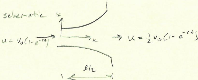
If  $V_0 = 10 \text{ ft/s}$  and  $l = 5 \text{ ft}$  determine  $c$  (other than  $c=0$ ) is needed to make the acceleration zero for any  $x$  at  $t=1 \text{ s}$ . Find expression for  $c$
