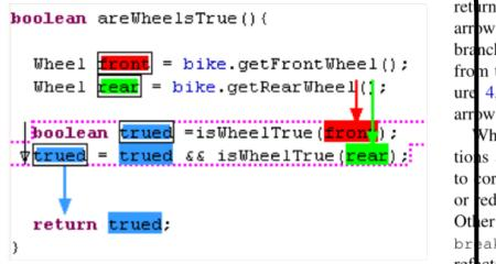
Fig. 3. Refactoring Annotations overlaid on program text. The programmer has selected two lines (between the dotted lines) to extract. Refactoring Annotations show how the variables will be used: front and rear will be parameters, as indicated by the arrows into the code to be extracted, and trued will be returned, as indicated by the arrow out of the code to be extracted.
