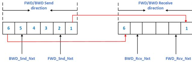
**Figure 4: Left: Transmit window at the sender. Right: Receive window at the receiver. Each window accommodates 6 packets. FBDT sender transmits packets for both forward and backward directions. The pointers showing the next forward and backward packets to be served are also illustrated.**
