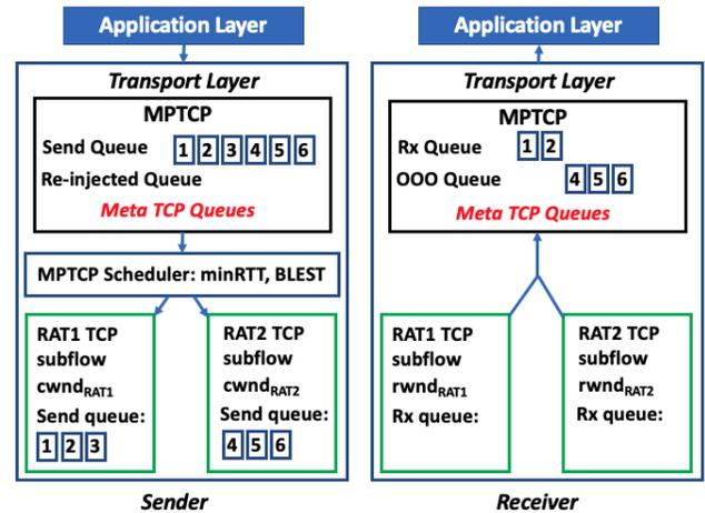
**Figure 2: MPTCP architecture. Packet 3 from RAT1 is lost. Packets 4, 5, and 6 are received at the receiver but moved to the out-of-order buffer. The loss stops subsequent packet deliveries to the Meta Rx queue and the application.**
