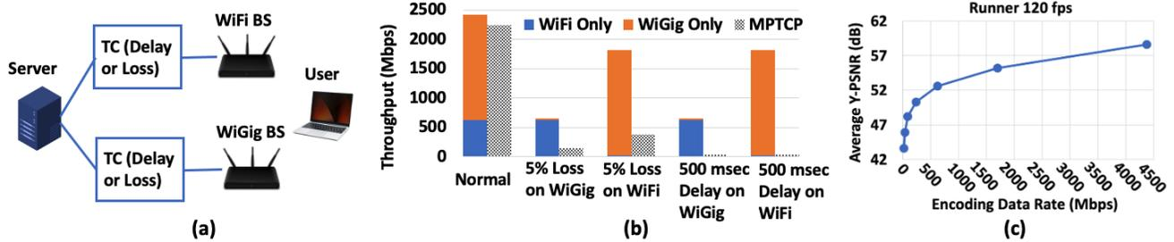
Figure 3: (a): We conduct experiments leveraging two Netgear Nighthawk X10 routers, a Dell Server and an Acer TravelMate laptop; (b): Throughput comparison of MPTCP’s default scheduler (BLEST) and individual SPTCP throughput under ideal, lossy, and delay induced scenarios. Similar drop in performance was observed with minRTT scheduler; (c): Trade-off between delivered 360° video quality and required minimum transmission data rate.
