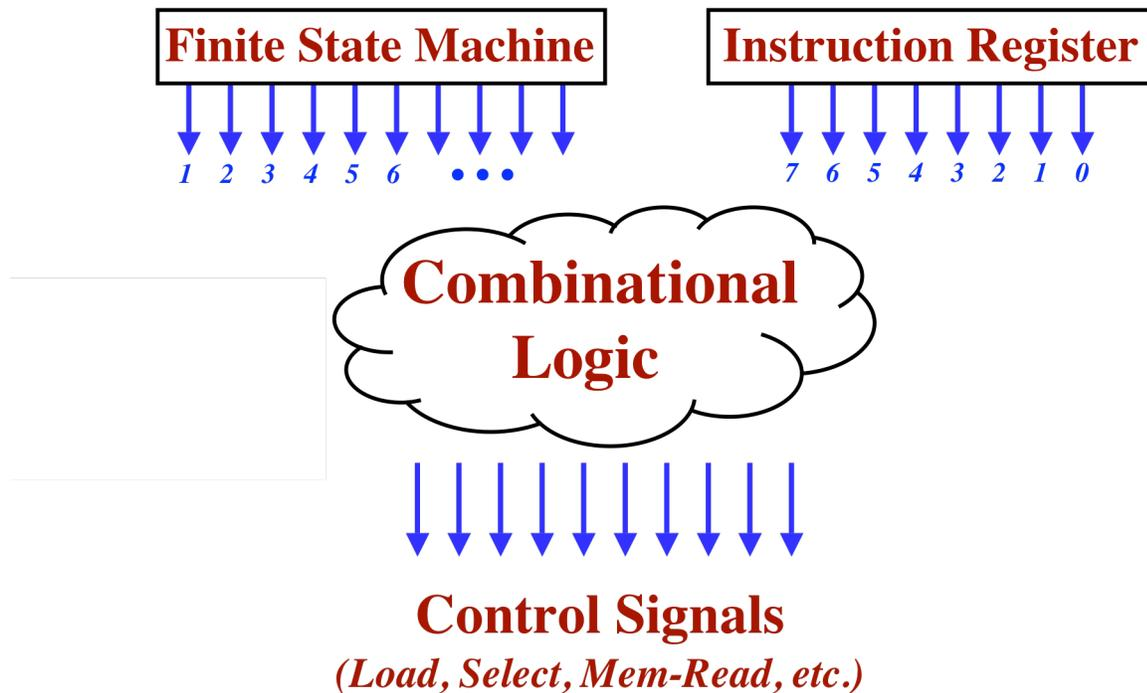
Connecting the inputs to the outputs, we have some “combinational logic”. Combinational logic is functional, in the sense that the outputs depend only on the inputs. There is no state. Any combinational logic can be constructed using simple logic gates such as AND, OR, and NOT and we know even how to design and optimize combinational circuitry automatically.
