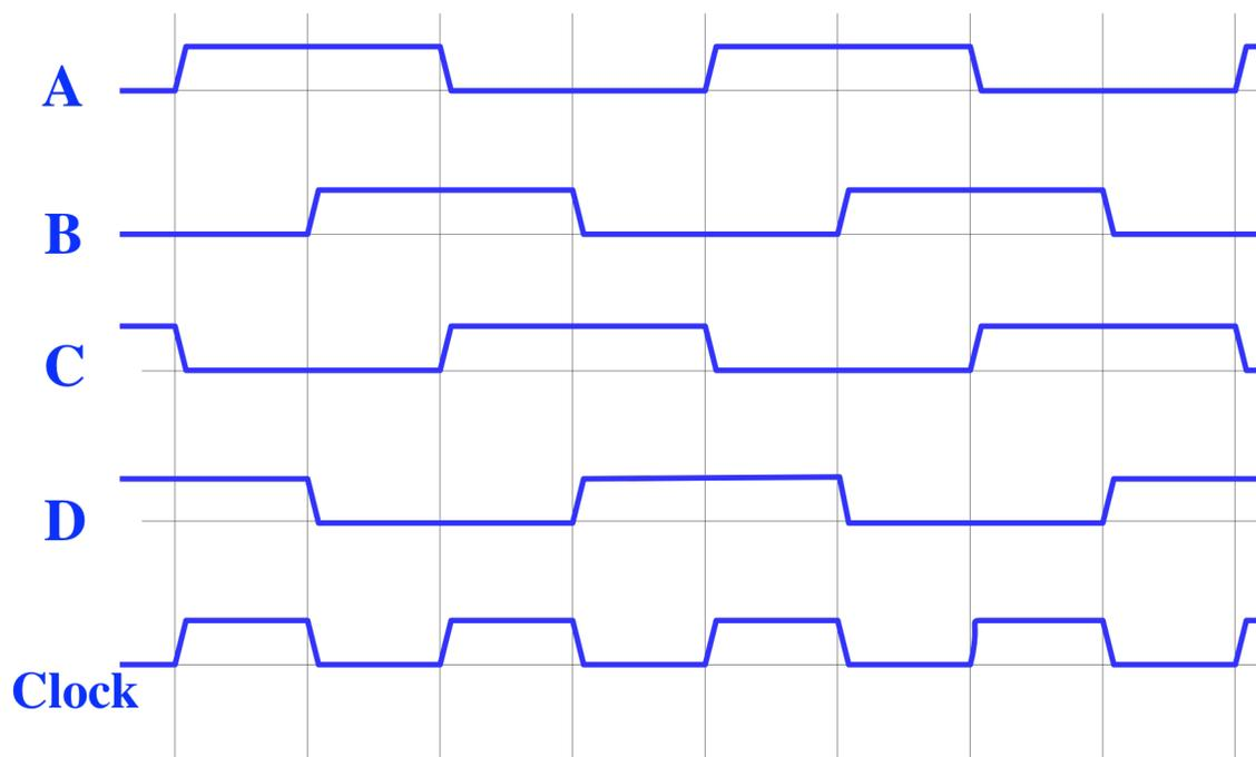
Note that each relay stays on for 2 units of time. During the first time interval, power is supplied to it and its capacitor is charging. During the second interval, power has been cut (by the transition of the relay directly above it) and it stays on while its capacitor discharges.
