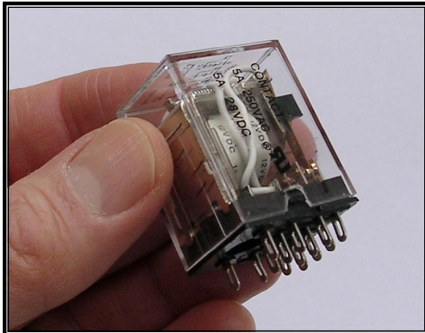
Incidentally, the term “computer bug” originated when a program failure was found to be caused by a moth, which had gotten caught between two contacts in an early relay-based computer. As you can see, these relays have a plastic cover, which makes this computer completely immune to “bugs.”
