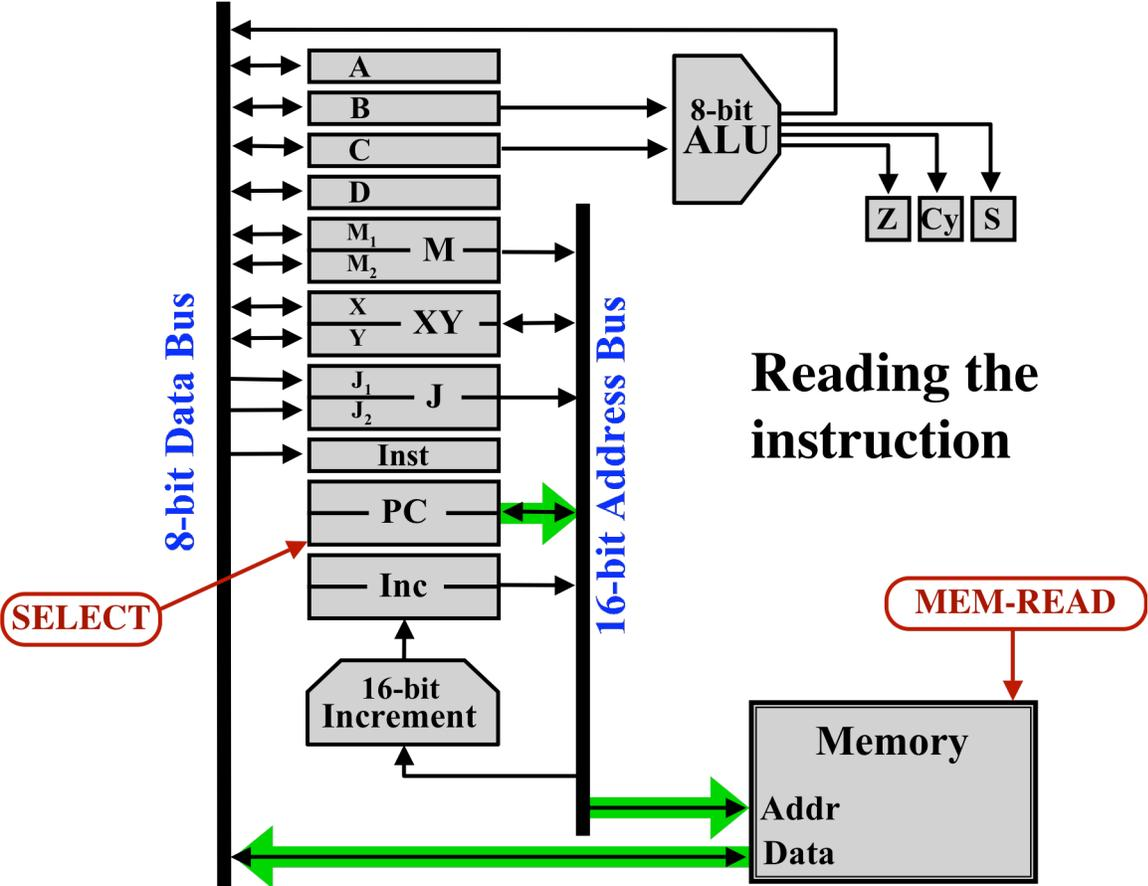
In the next step, the Load-Inst control line goes high, which causes the 8 bit instruction register to be loaded.
