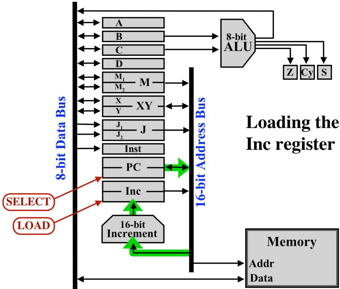
The second part of incrementing the PC is to copy the new value from the Inc register back to the PC. First the Inc register is gated onto the address bus. Then the Load-PC control line is asserted to load the PC register.
