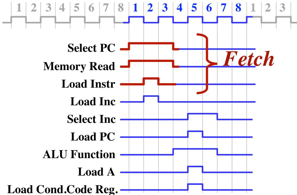
In the next timing diagram, the control signals associated with incrementing the PC are highlighted in red.
