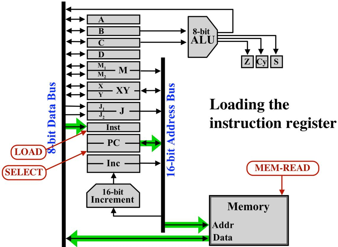
The Program Counter is always incremented at the beginning of each instruction. This takes two steps: first the “Inc Register” is loaded with the old value of the PC, plus one; then the new value is copied from the Inc Register back to the PC register. The first step can be overlapped with the fetching of the instruction from memory.
