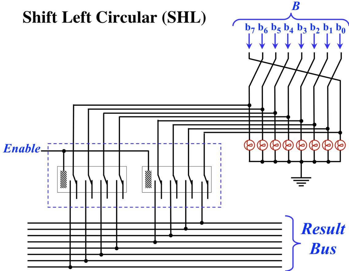
Sometimes a circular shift is called “rotate”. This computer can only shift by one bit and cannot shift right, but notice that you can achieve the effect of shifting right by one bit by shifting left 7 times. Therefore, a single “shift left” instruction is included in the instruction set, since any other shift amount can be achieved with up to 7 repetitions of the instruction.
