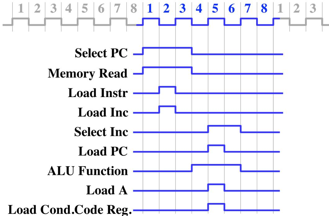
Each of these control lines has a switch on the front panel of the computer. Thus, you could manually execute the actions of an ADD instruction by flipping these control lines in exactly the order shown in this diagram.
