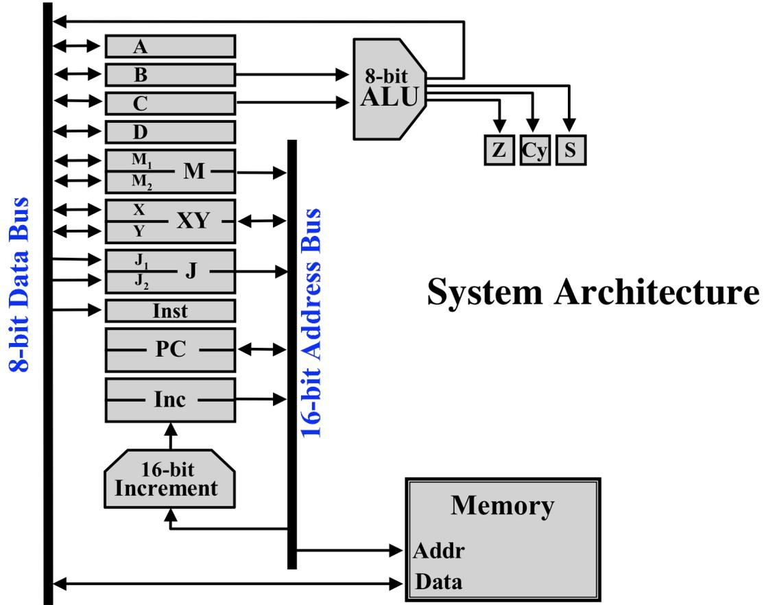
The 8-bit data bus is shown as a single heavy line, although there are of course 8 parallel wires. Likewise, the address bus is shown as a single line, instead of showing all 16 wires.
