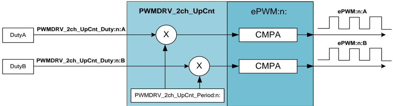
This macro is used in conjunction with the peripheral configuration file PWM\_2ch\_UpCnt\_Cnf.c. The file defines the function:
