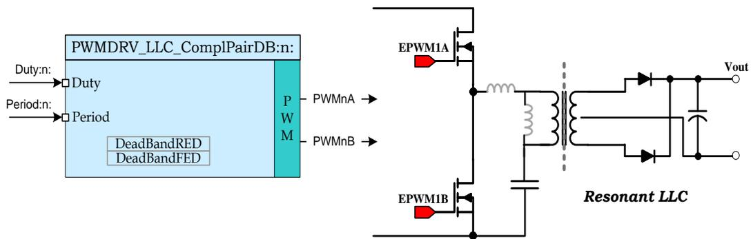
**Resonant LLC converter driven by PWMDRV\_LLC\_CmplPairDB module**
