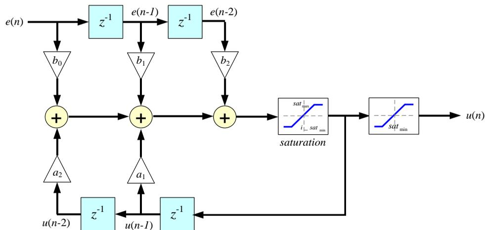
Input and output data are located in internal RAM with address designated by CNTL\_2P2Z\_DBUFF as shown below. Note that to preserve maximum resolution the module saves the values inside CNTL\_2P2Z\_DBUFF in `_IQ30` format.
