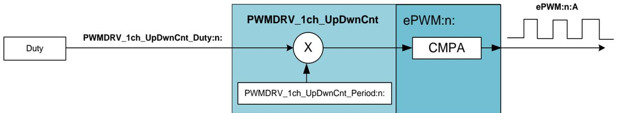
This macro is used in conjunction with the peripheral configuration file PWM\_1ch\_UpDwnCnt\_Cnf.c. The file defines the function
