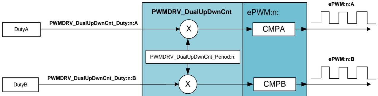
This macro is used in conjunction with the peripheral configuration file PWM\_DualUpDwnCnt\_Cnf.c. The file defines the function
