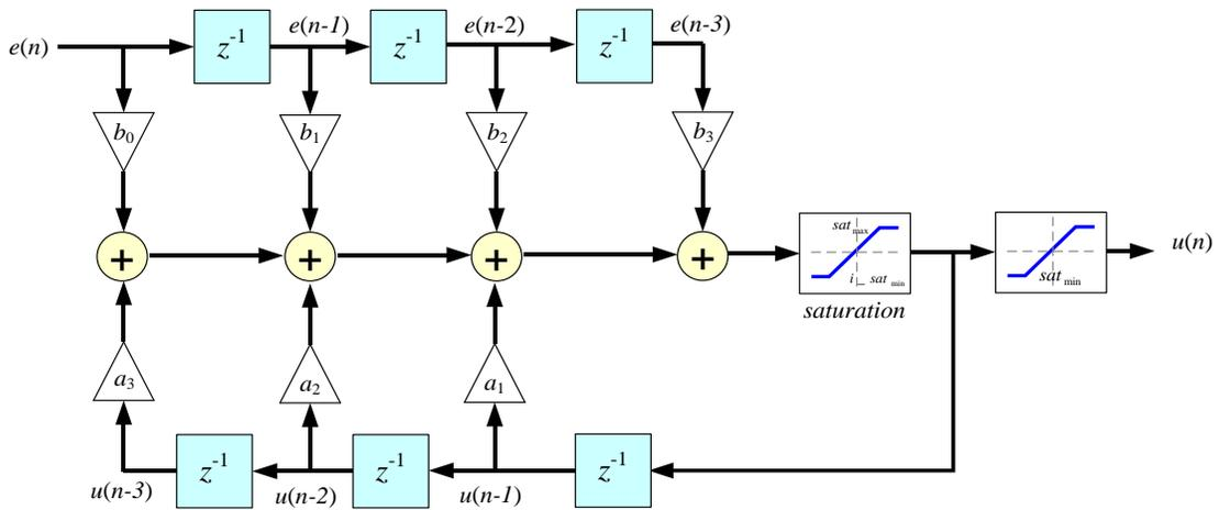
Input and output data are located in internal RAM with address designated by CNTL\_3P3Z\_DBUFF as shown below. Note that to preserve maximum resolution the module saves the values inside CNTL\_3P3Z\_DBUFF in \_IQ30 format.
