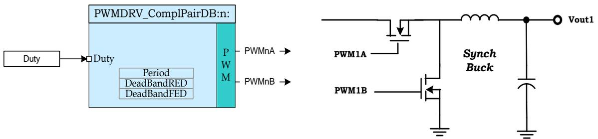
**Synchronous Buck converter driven by `PWMDRV_CmplPairDB` module**
