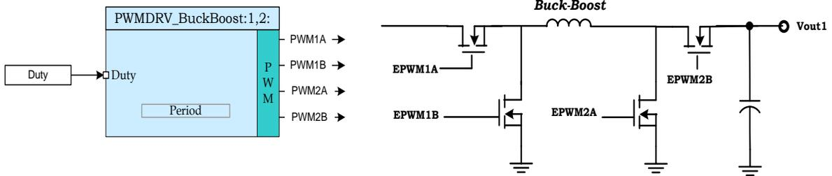
***Buck Boost Converter driven by PWMDRV\_BuckBoost module***
