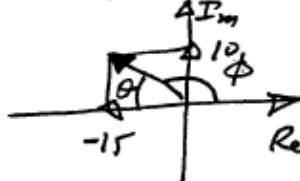
$$\phi(\omega) = -[180^\circ - 10^\circ] = [180^\circ - \tan^{-1} \frac{10}{15}] = -146.3^\circ$$
