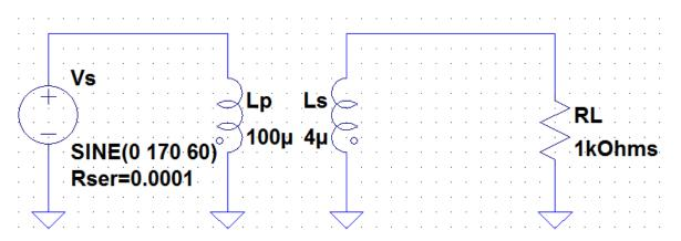
This transformer won't work properly because LTSpice does not know this is a transformer. This looks like two inductors are in the circuit. We need to tell LTSpice these are transformer. We
