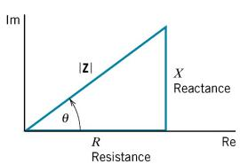
where  $R = \text{Re}(\mathbf{Z})$  is the resistance and  $X = \text{Im}(\mathbf{Z})$  is the reactance. Positive X is for L (or lagging) and negative X is for C (or leading).
