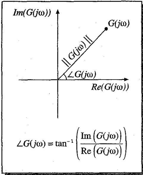
$$G(j\omega) = \frac{1}{1 + j \frac{\omega}{\omega_0}} = \frac{1 - j \frac{\omega}{\omega_0}}{1 + \left(\frac{\omega}{\omega_0}\right)^2}$$
