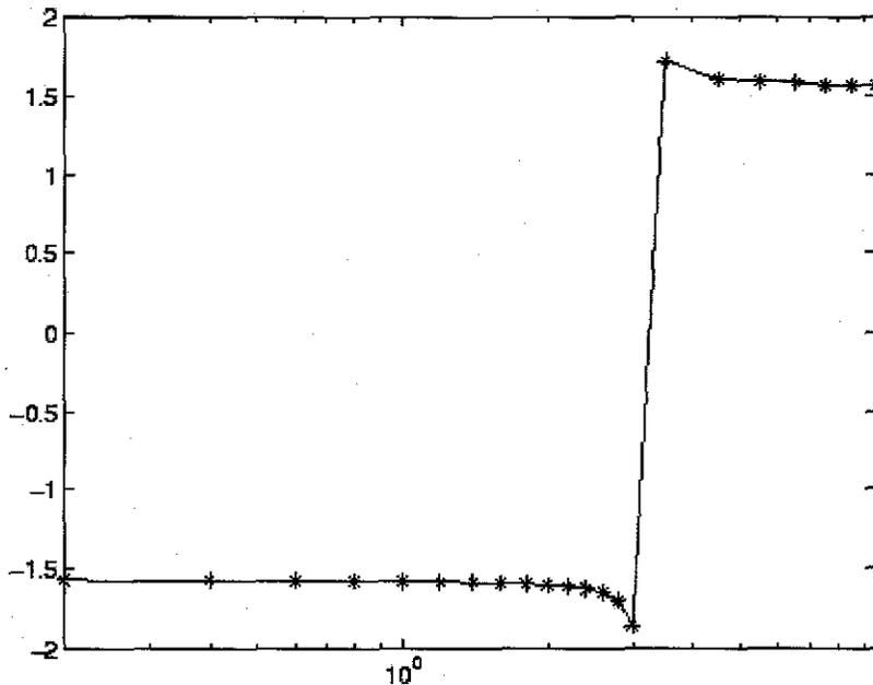
Using `unwrap` to correct the phase angle, the resulting jump is 2.6959, which is less than the default jump tolerance  $\pi$ . This figure plots the new curve over the original curve.
