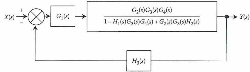
Similarly, by applying transforms 1 and 3 we obtain the simplified block diagram that represents the system's transfer function.
