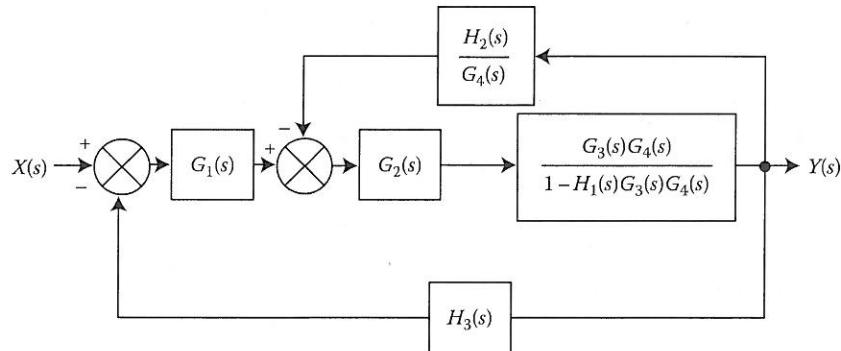
Next we apply transformations 1 and 3 to the loop that contains the transfer function  $H_2(s)/G_4(s)$  as feedback and get the following block diagram:
