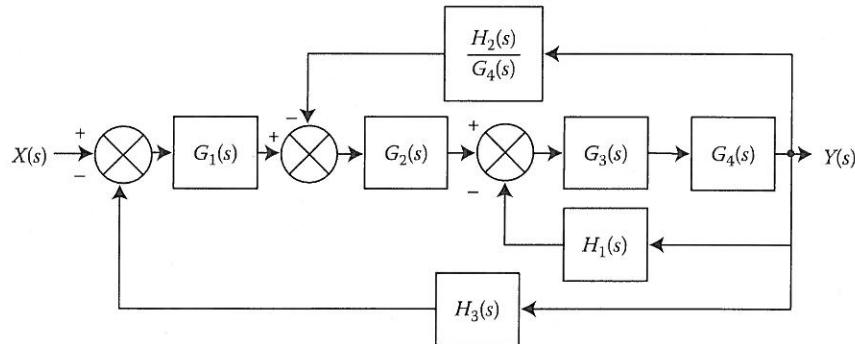
The next block diagram emerges when transformations 1 and 3 are applied to the loop that contains the blocks with transfer functions  $G_3(s)$ ,  $G_4(s)$ , and  $H_1(s)$ .
