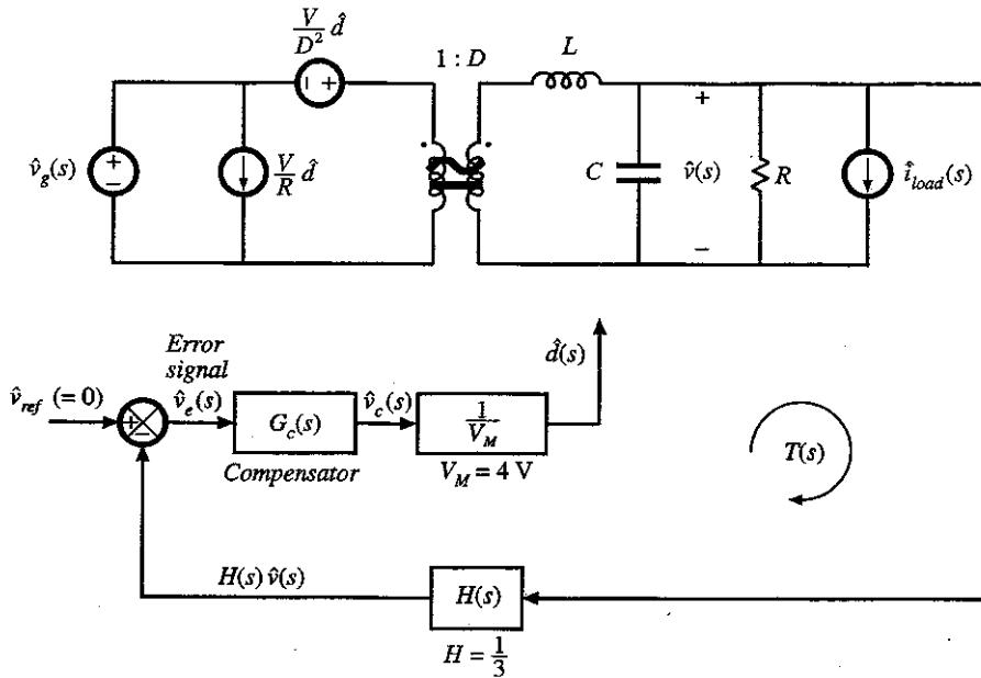
Open-loop control-to-output transfer function  $G_{vd}(s)$
