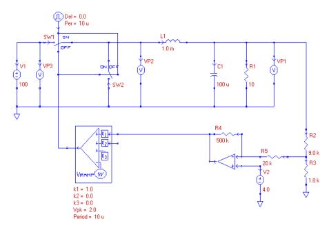
The parameters of the Buck regulator are:  $V_g = 100V$ ,  $V_{out} = 40V$ ,  $L=1 \ mH$ ,  $C=100 \ \mu F$ ,  $V_M = 2V (V_M$  is the peak-to-peak amplitude of the sawtooth waveform used in the Pulse Width Modulator (*PWM*), and  $f_s = 100kHz$ . The reference voltage used is  $V_{ref} = 4 V$ .
