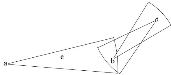
a sends a tone to  $b$  but  $b$  is busy receiving a packet from  $d$ . However,  $c$  responds leading to an unnecessary transmission from  $a$  that may interfere at  $b$ .
