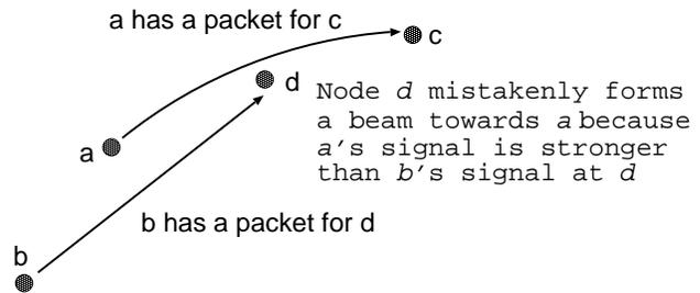
Fig. 1. False beamforming.
