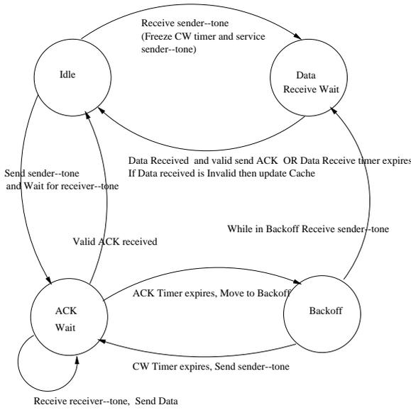
Fig. 4. State diagram of the Tone-based 802.11b protocol.
