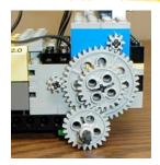
Use gears to slow down your robot. Gears also give your robot more strength (torque). The wheel spins 5 times slower than the motor.
