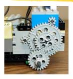
The total gear ratio is... (5 / 1) x (1 / 1) = 5 to 1.
