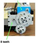
It takes 5 revolutions of the 8 tooth gear to make the 40 tooth gear go around once.
