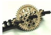
Idler gears **DO NOT** change the gear ratio.
