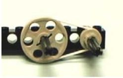
Unlike gears, the pulleys rotate in the **same** direction.
