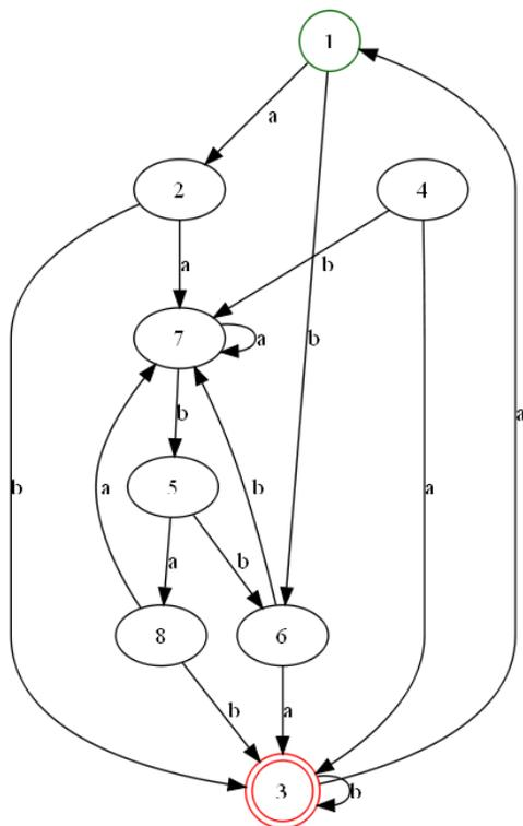
Note: the start state is state 1. This machine generated graph indicates start states with green circles.
