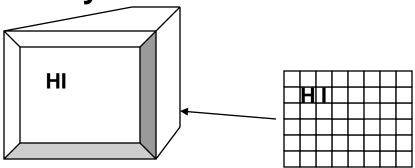
Buffered graphics use two sets of memory, instantaneously switching from one memory to the other, so quickly that the flicker effect is unobservable.
