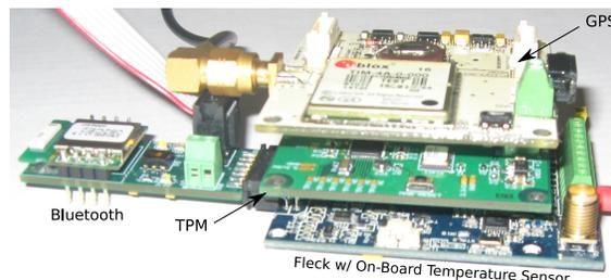
Figure 2: Trusted sensing peripheral with GPS sensor
