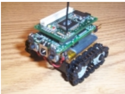
Figure: The Robomote: a mobile sensor node End Box 2
