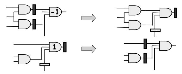
A negative latch has the interpretation that it advances its input by 1 clock cycle instead of delaying it by one clock cycle 21
