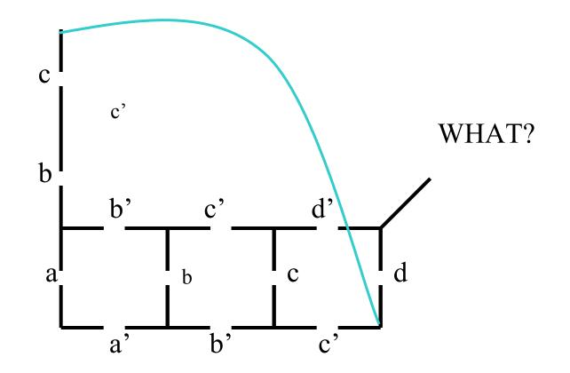
The symmetric function can be mapped in to the lattice of multiplexers as shown in the figure below. Can you prove that by replacing multiplexers with ARBITRARY other gates we will be able still to realize arbitrary symmetric function. Control variables of multiplexers are not shown here.
