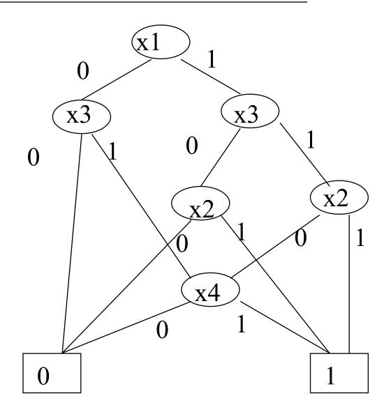
Realize the function expressed by this lattice diagram using only 2-input gates (arbitrary). Minimize the number of used gates. Draw a Kmap of this function and verify your solution.
