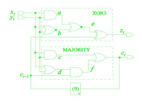
In this view the gates of the full adder circuit are just logic equations
