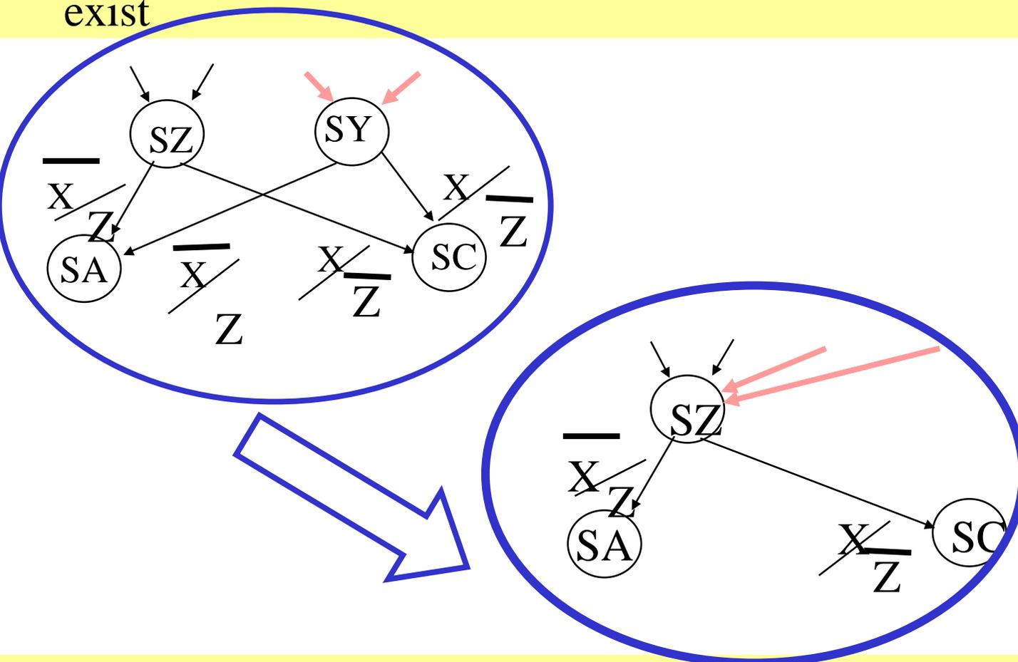
States SZ and SY are equivalent and are combined to one state by pointing all arrows that go to SY to state SZ and removing SY with its all arrows
