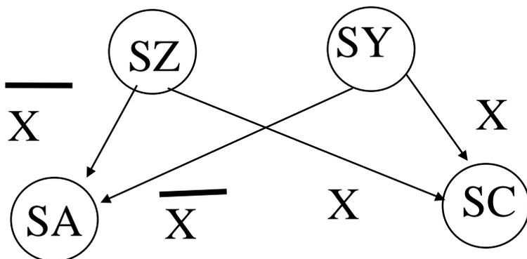
States SY and SZ are equivalent and are combined to one state by pointing all arrows that go to SY to state SZ and removing SY with its all arrows
