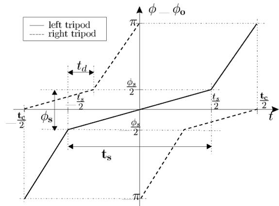
Figure 9: Motion profiles for left and right tripods.
