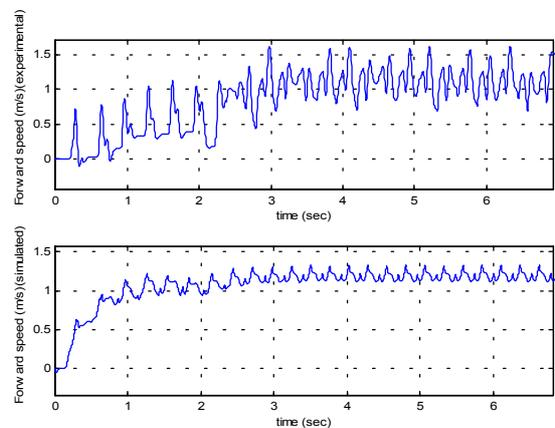
Figure 5: Forward velocity. Top: Experiment. Bottom: Simulation.
