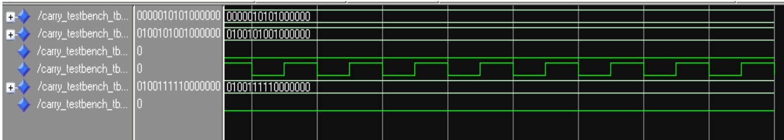
The simulation result shows the output 16 bit vector of (010011110000000) when the two inputs are  $x_i = 0000010101000000$  and  $y_i = 0100101001000000$ .
