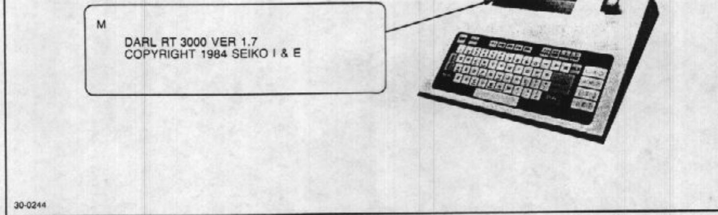
*Figure 3.16 Teach-Terminal LCD Message at Power "ON"*
