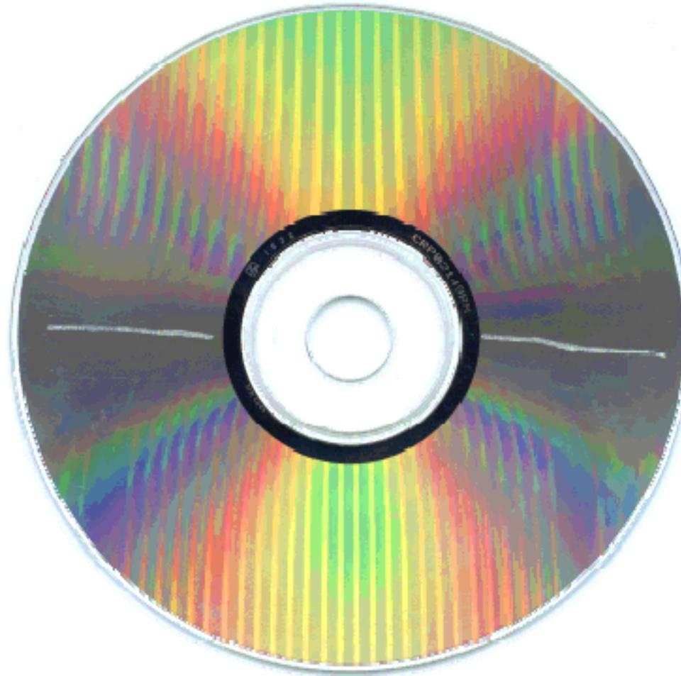
This deliberately-damaged CD can be read without errors
