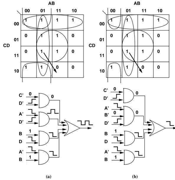
Figure 6: Combinational hazard example: dynamic MIC transition
