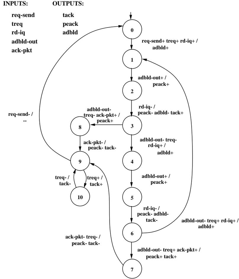
Figure 12: Burst-mode specification for HP controller *pe-send-ifc*
