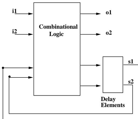
Figure 10: Block diagram of a Huffman machine
