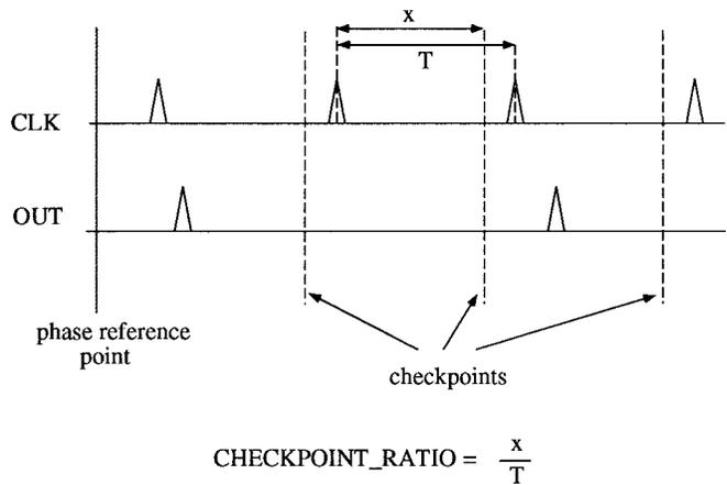
Fig. 3. *MALT*: Generating pass–fail criteria for *synchronous* circuits. Positions of checkpoints are determined on the basis of the CHECKPOINT\_RATIO, which defines the relative position of each checkpoint in the clock cycle.
