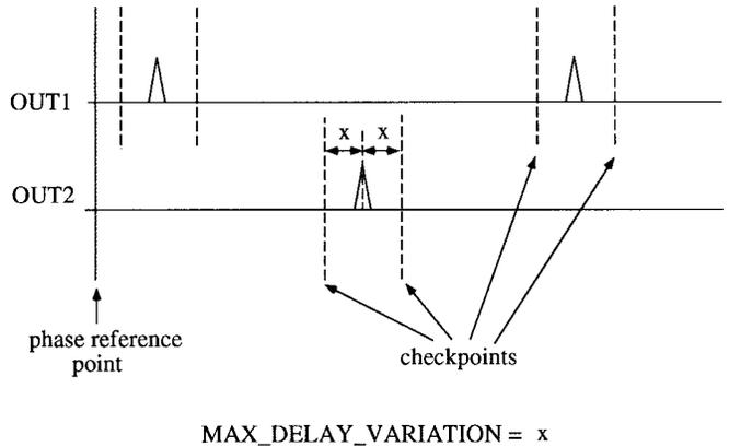
Fig. 4. MALT: Generating pass-fail criteria for *asynchronous* circuits. Positions of checkpoints are determined on the basis of MAX\_DELAY\_VARIATION, which determines the distance between each checkpoint and a nominal position of an SFQ pulse at the output of the circuit.
