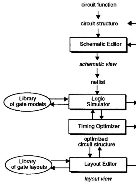
Fig. 2. Design flow for large-scale superconducting digital circuits.
