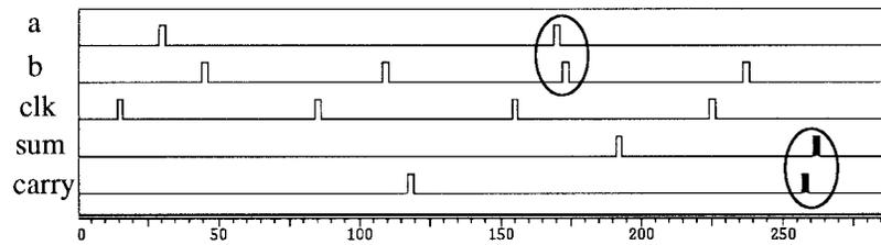
Fig. 6. HDL: Verilog-XL simulation of an RSFQ half-adder;  $sum = a \oplus b$ ,  $carry = a \cdot b$ . Shaded pulses at the  $sum$  and  $carry$  output in the fourth clock cycle depict the violation of the minimum separation time between the pulses at the inputs  $a$  and  $b$  in the previous clock cycle.
