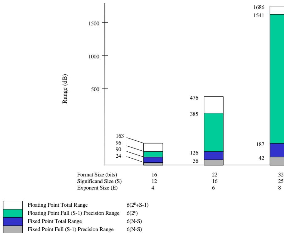
**Figure 7: Floating-point format comparisons.**
