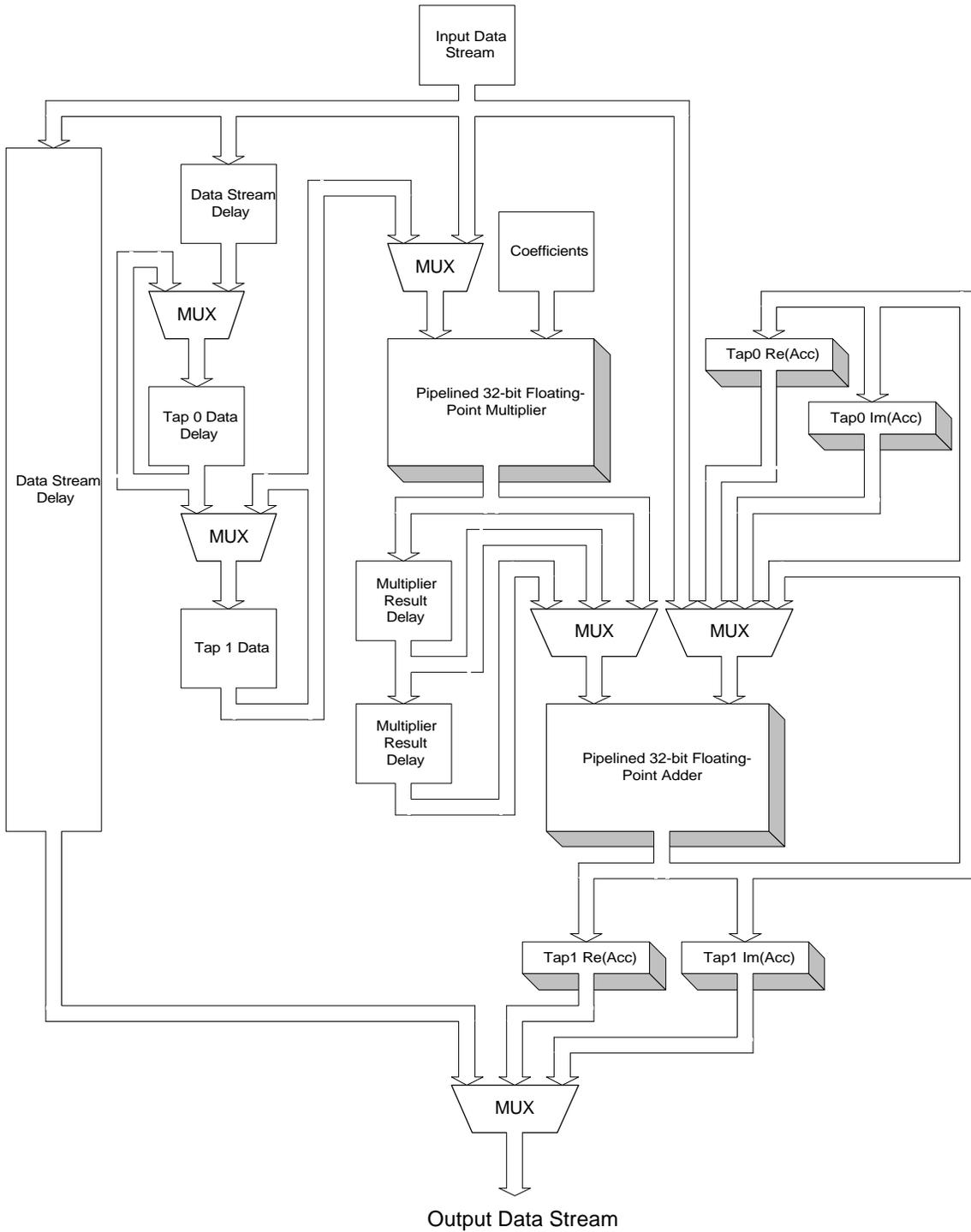
**Figure 15: Processing element component connectivity.**
