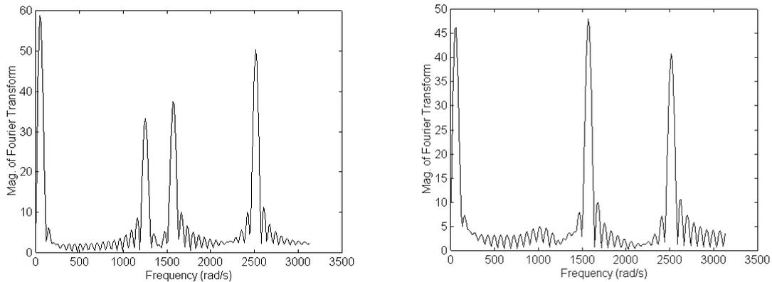
**Figure 40: Bandstop filtered signal spectrums for 7-tap (left) and 31-tap (right) filters.**
