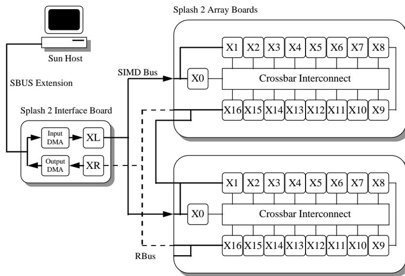
**Figure 5: Two board Splash system.**
