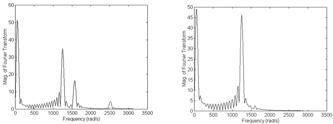
**Figure 31: Lowpass filtered signal spectrums for 7-tap (left) and 31-tap (right) filters with a target cutoff frequency of 1413.7 rad/s (225 Hz).**
