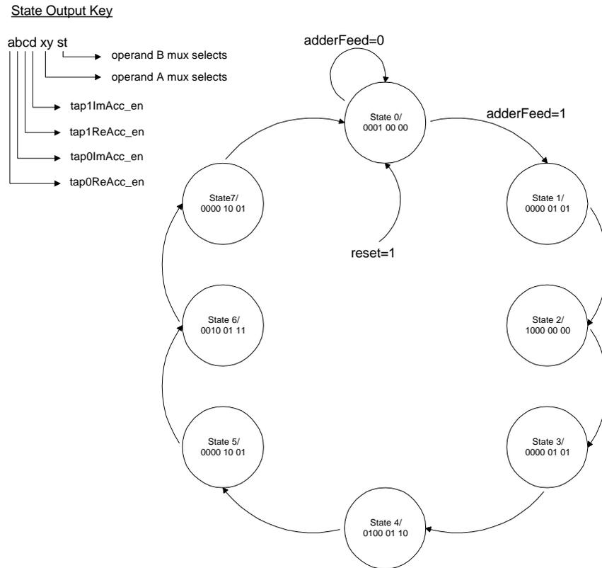
**Figure 29: Adder operand feeding finite state machine.**
