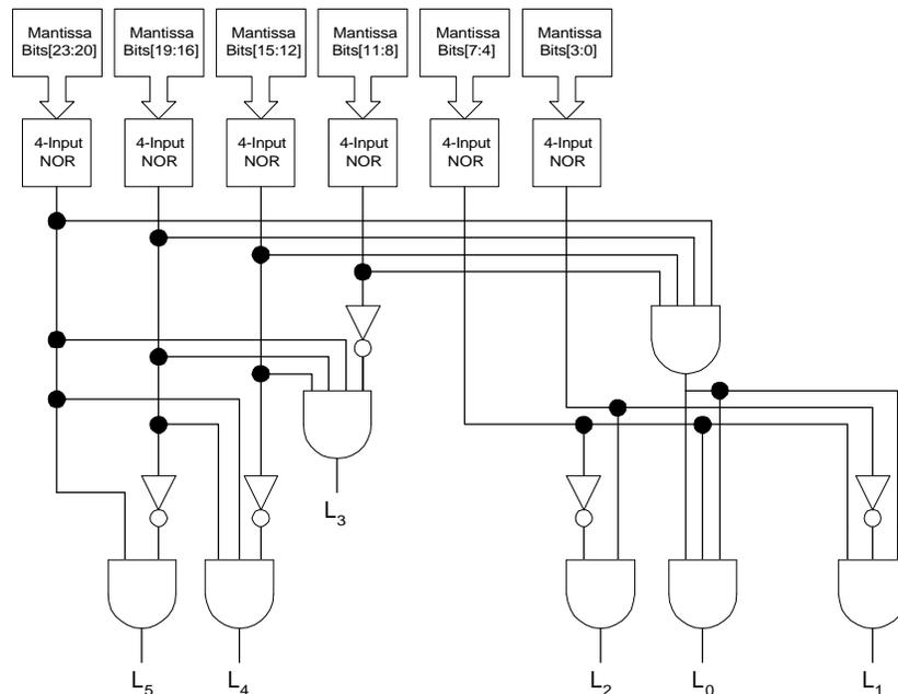
**Figure 11: Leading-one detection logic.**
