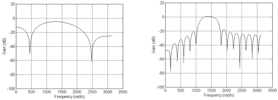
**Figure 36: Bandpass filter frequency responses for 7-tap (left) and 31-tap (right) filters with a target cutoff frequency of 1130.97 rad/s (180 Hz) and 1696.46 rad/s (270 Hz).**
