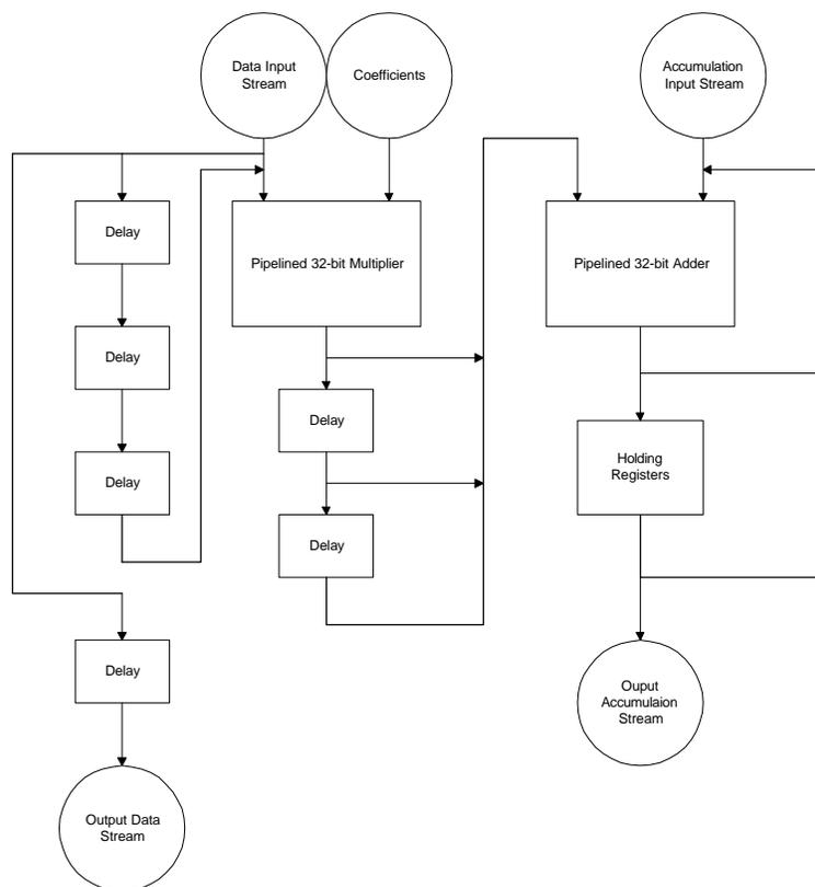
**Figure 18: Processing element internal data flow paths.**
