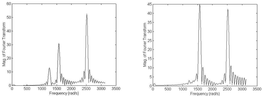
**Figure 34: Highpass filtered signal spectrums for 7-tap (left) and 31-tap (right) filters.**
