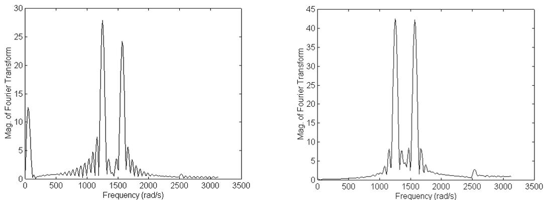
**Figure 23: Spectrum plot of bandpass filtering for 7 taps (left) and 31 taps (right).**
