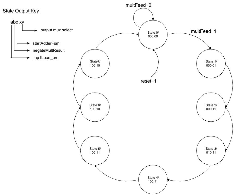
**Figure 28: Multiplier loading finite state machine.**
