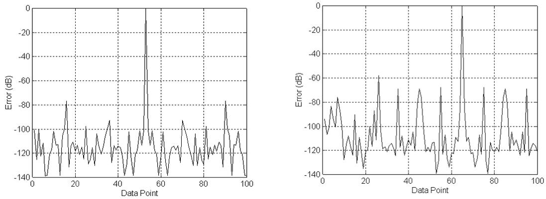
**Figure 38: Bandpass filter output error analysis for 7-tap (left) and 31-tap (right) filters.**
