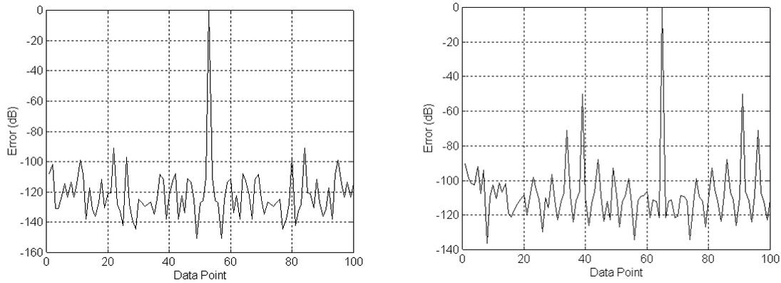
**Figure 32: Lowpass filter output error analysis for 7-tap (left) and 31-tap (right) filters.**
