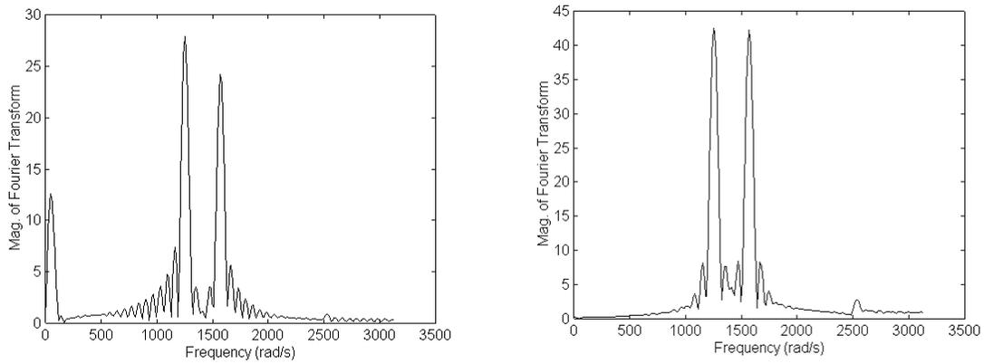
**Figure 37: Bandpass filtered signal spectrums for 7-tap (left) and 31-tap (right) filters.**
