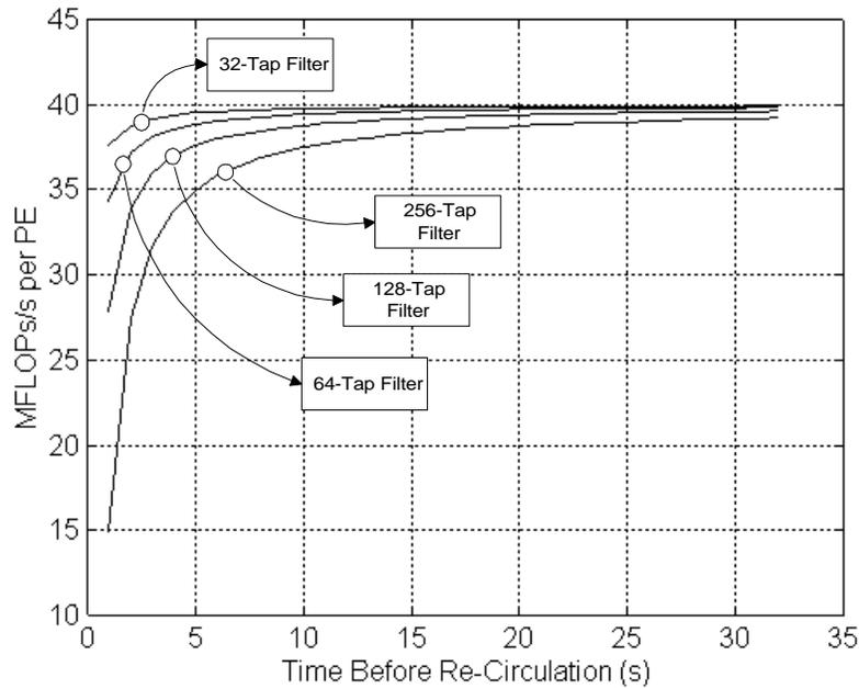
**Figure 25: Effective filter performance with data re-circulation.**
