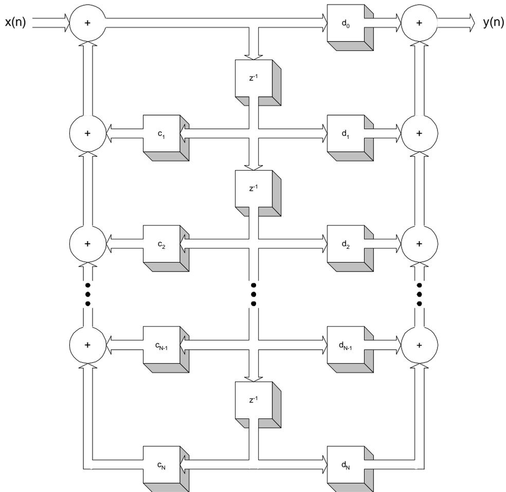
**Figure 2: Direct Form II realization signal flow graph of an IIR.**
