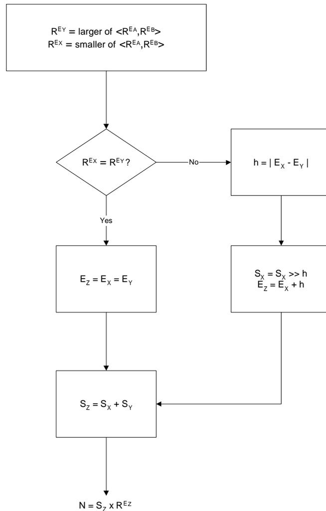
**Figure 9: Flow diagram for floating-point addition.**
