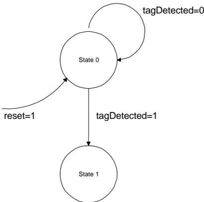
**Figure 26: Data detection finite state machine.**
