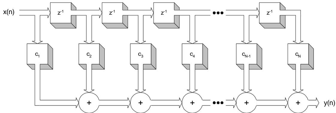
**Figure 3: Direct Form realization signal flow graph of an FIR.**
