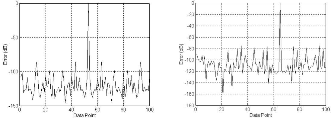
**Figure 35: Highpass filter output error analysis for 7-tap (left) and 31-tap (right) filters.**
