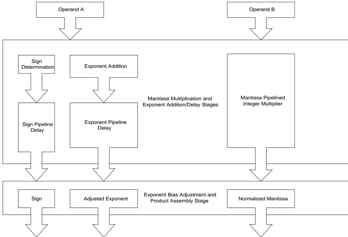
**Figure 12: Pipelined Multiplier Block Diagram.**
