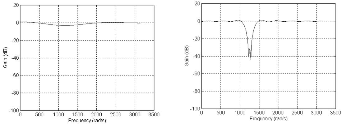
**Figure 39: Bandstop filter frequency responses for 7-tap (left) and 31-tap (right) filters with a target cutoff frequency of 1130.97 rad/s (180 Hz) and 1382.30 rad/s (220 Hz).**
