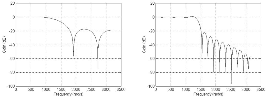
**Figure 30: Lowpass filter frequency responses for 7-tap (left) and 31-tap (right) filters with a target cutoff frequency of 1413.7 rad/s (225 Hz).**
