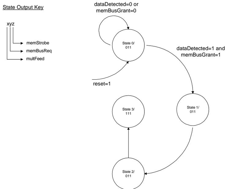
**Figure 27: Coefficient loading finite state machine.**
