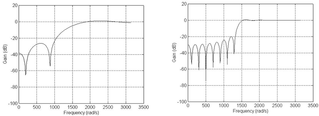
**Figure 33: Highpass filter frequency responses for 7-tap (left) and 31-tap (right) filters with a target cutoff frequency of 1413.7 rad/s (225 Hz).**
