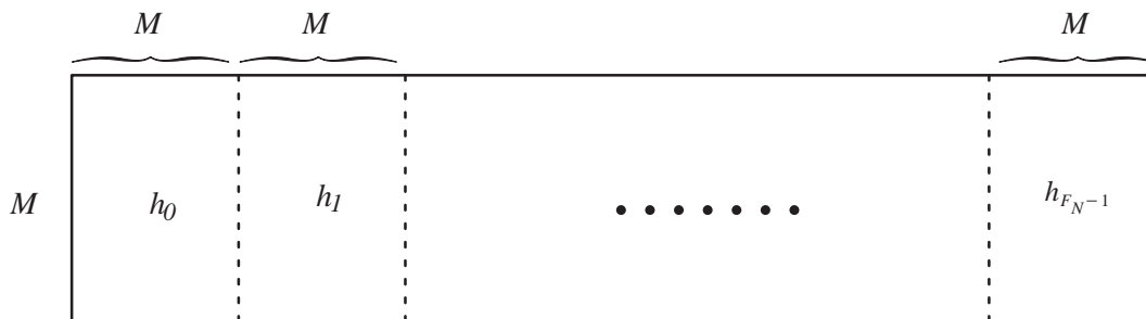
Figure 3–3: Construction of Matrix A with Multiple Orientational Filters
