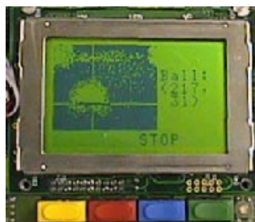
Figure 25. LCD output after ball detection
