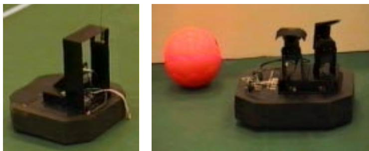
Figure 74. Alpha plus Alpha - common field player and modified goal keeper robot with two cameras
