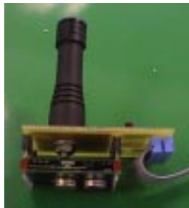
Figure 12. Wireless communication module
