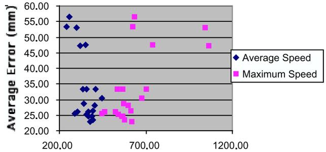
Figure 9: Avg. Error vs Speed (10 Pixel Lookahead Distance)
