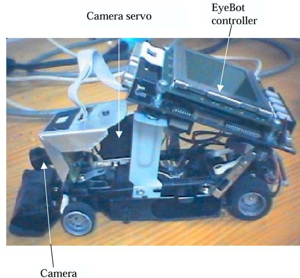
Figure 1: Local Vision Autonomous Robot Platform
