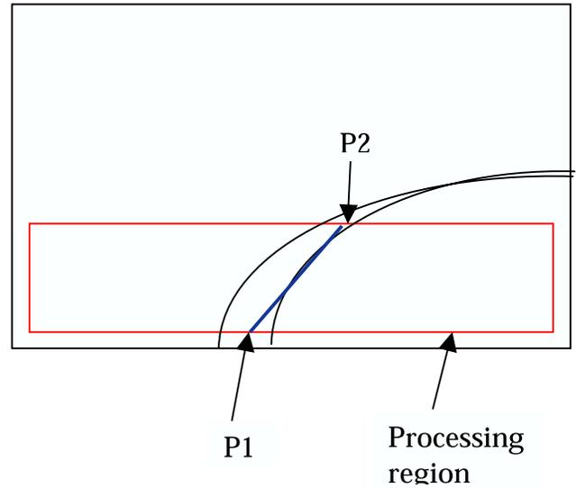
Figure 3: Determining the Offset And Gradient From the Image. Only the boundary of the region is processed.
