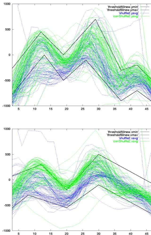
Figure 5: Corrected and uncorrected dynamic walking gait in the sagittal (top) and lateral (bottom) plane.
