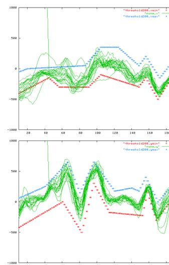
Figure 3: Gyroscope Readings in the lateral and saggital plane over 10 Steps. Linear Approximation of the Safe Zone.
