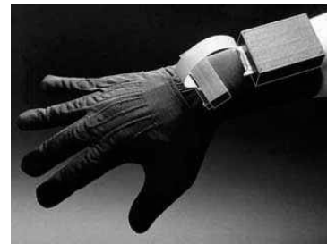
Optical fibres measure bend of the finger
