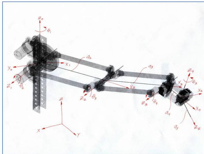
Figure 5: Reference frames based on Denavit-Hartenberg representation.
