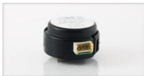
Encoders are installed on the two motors used on the robot. These encoders are made by US Digital. They are used to allow position control of the motors so they can perform similar to servos. The encoders used are optical quadrature encoders. These encoders use two output channels (A and B) to sense position. Using two code tracks
