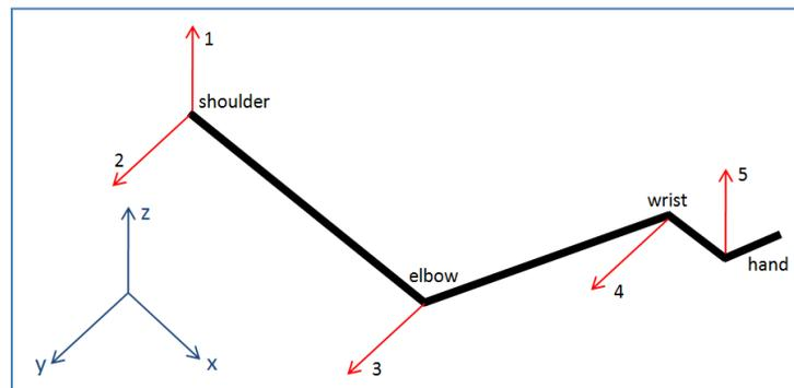
Figure 1: Robot arm's degrees of freedom.
