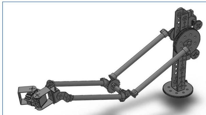
*Figure 3: Solid model of robot arm and hand assembly.*
