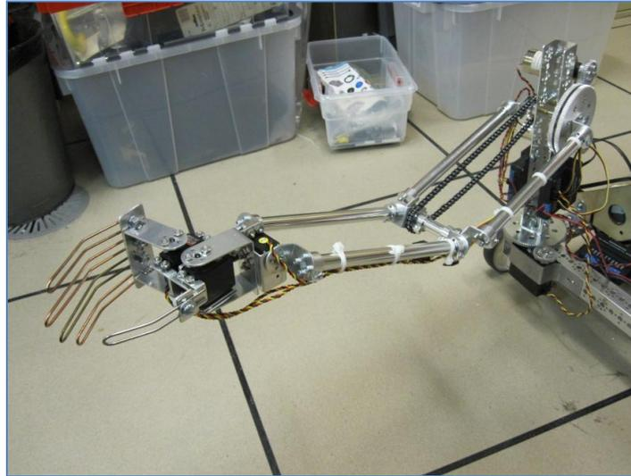
*Figure 4: Final TETRIX robot arm and hand assembly.*
