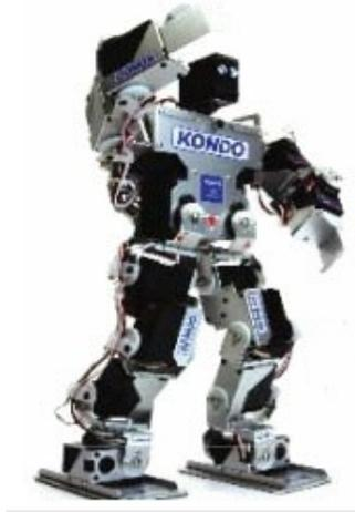
*Figure 5.25: Kondo KHR-1 humanoid robot<sup>20</sup>.*
