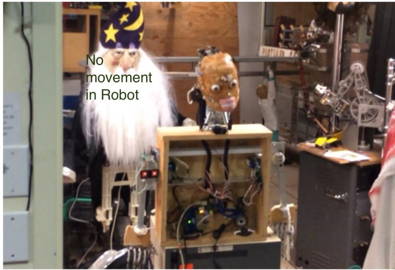
No person in the Kinect range, hence there is no movement in the robot arm
