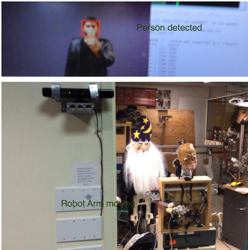
Person in the Kinect range, Facedetect program detects the person with red square displayed on the output screen and the movement in the robot arm is see
