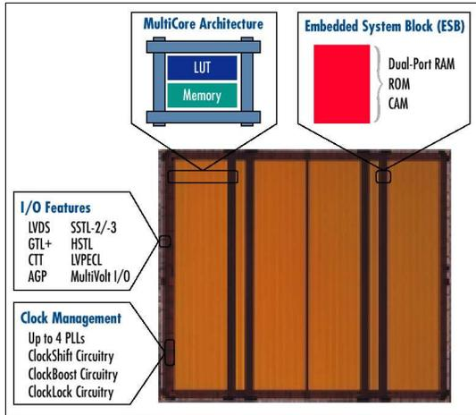
Figure 1: APEX Device Features
