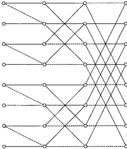
Figure 1. Fast butterfly diagram for forward Arithmetic-Walsh transform,  $n = 3$  and  $r = 2$ .
