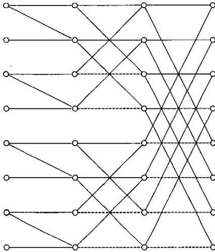
Figure 2. Fast butterfly diagram for inverse Arithmetic-Walsh transform,  $n = 3$  and  $r = 2$ .
