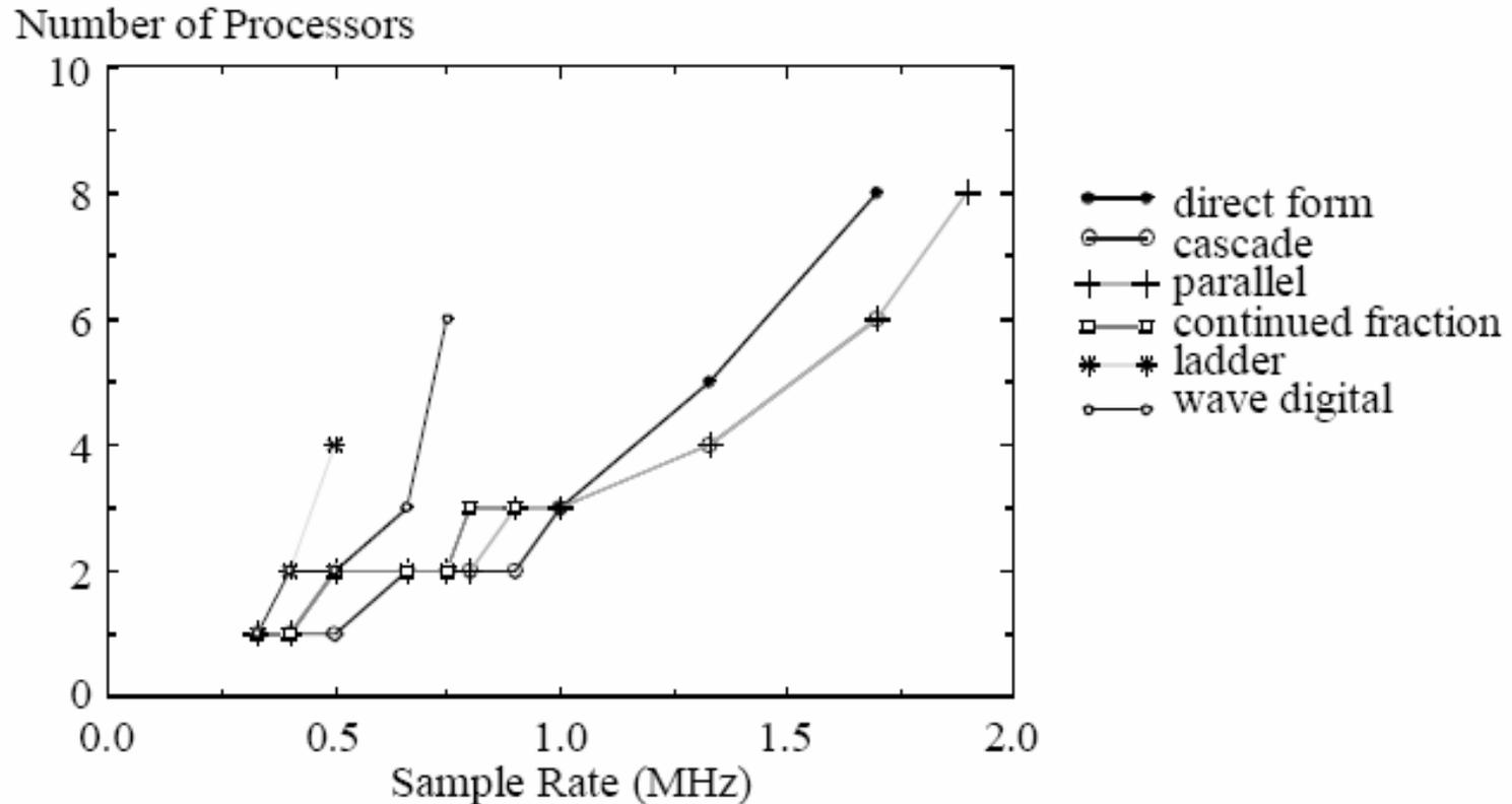
Fig. 32. Number of processors versus sample rate for 24-bit ALU implementations.
