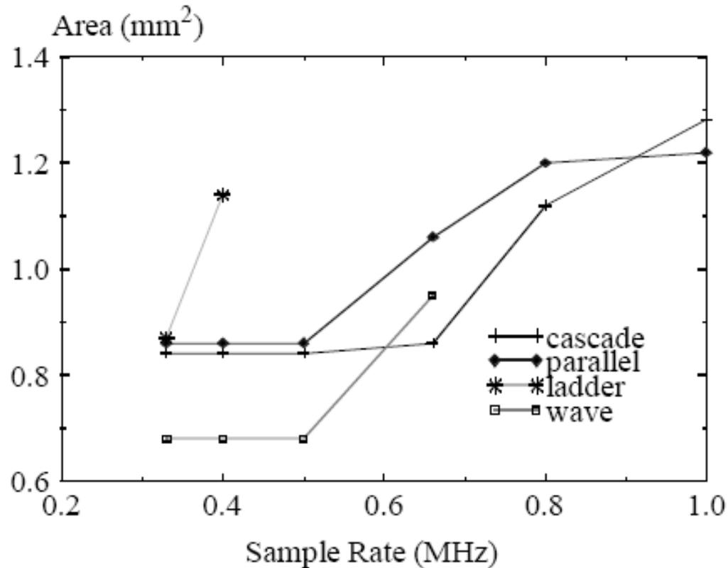
Fig. 33. Area for semi-custom ASIC implementations after constant multiplication expansion into additions and shifts.
