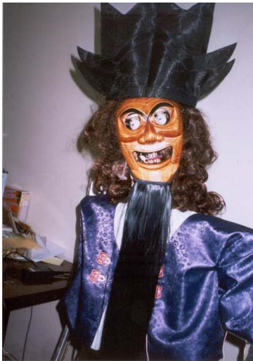
Figure 2. Sonbi the Confucian Scholar robot. Note eyes enlargement to make the eye movement more visible. There are color LEDs in the eyes.
