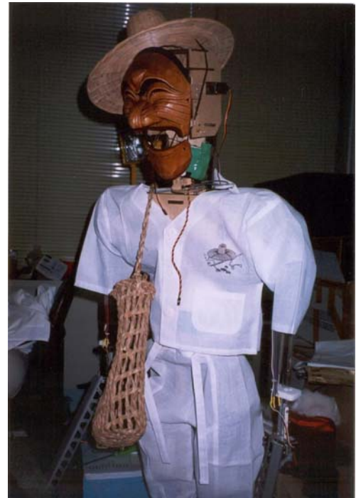
Figure 1. Paekchong the bad butcher robot. Note the moveable jaw
