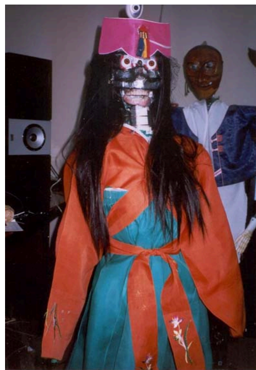
Figure 3. Kyng Jin Lee robot without skin. Please note the sensors on cheeks and nose and a camera on top of the head.
