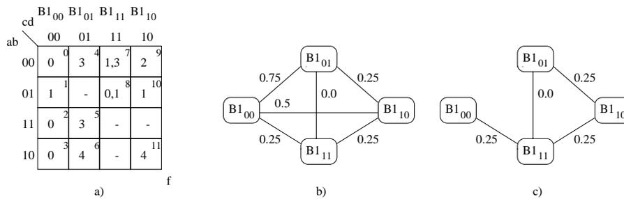
Figure 12: Compatibility graph construction for data with noise
